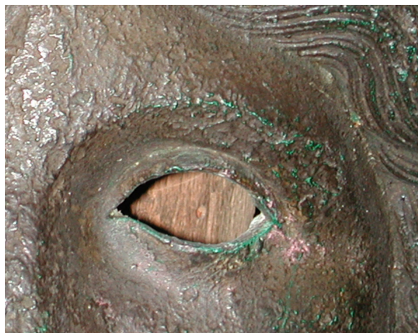
FIGURE 6.5. Detail photograph taken before disassembly of the statue, showing the internal wood support visible through the aperture of the left eye, along with details of the dark brown surface
