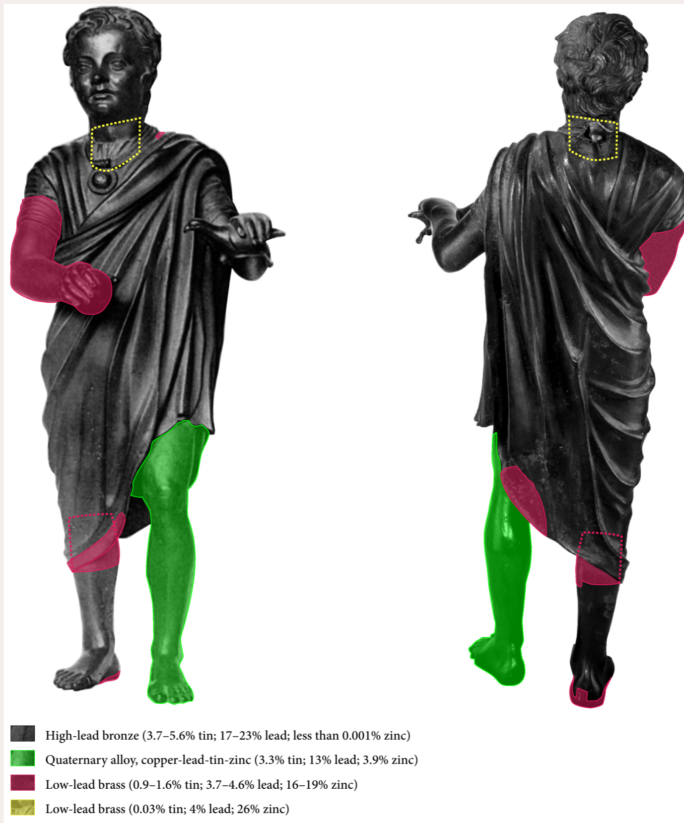
FIGURE 7.7. Cartographic representation of the statue: the different copper alloys. Gray: the ancient leaded bronze. Green: the quaternary alloy of the first phase of restoration (late sixteenth or seventeenth century). Pink: the leaded brass of the second phase of restoration (eighteenth century). Yellow dashed line: the leaded brass used to make a cylinder that was inserted in the neck during the restoration carried out between 1944 and 1964
