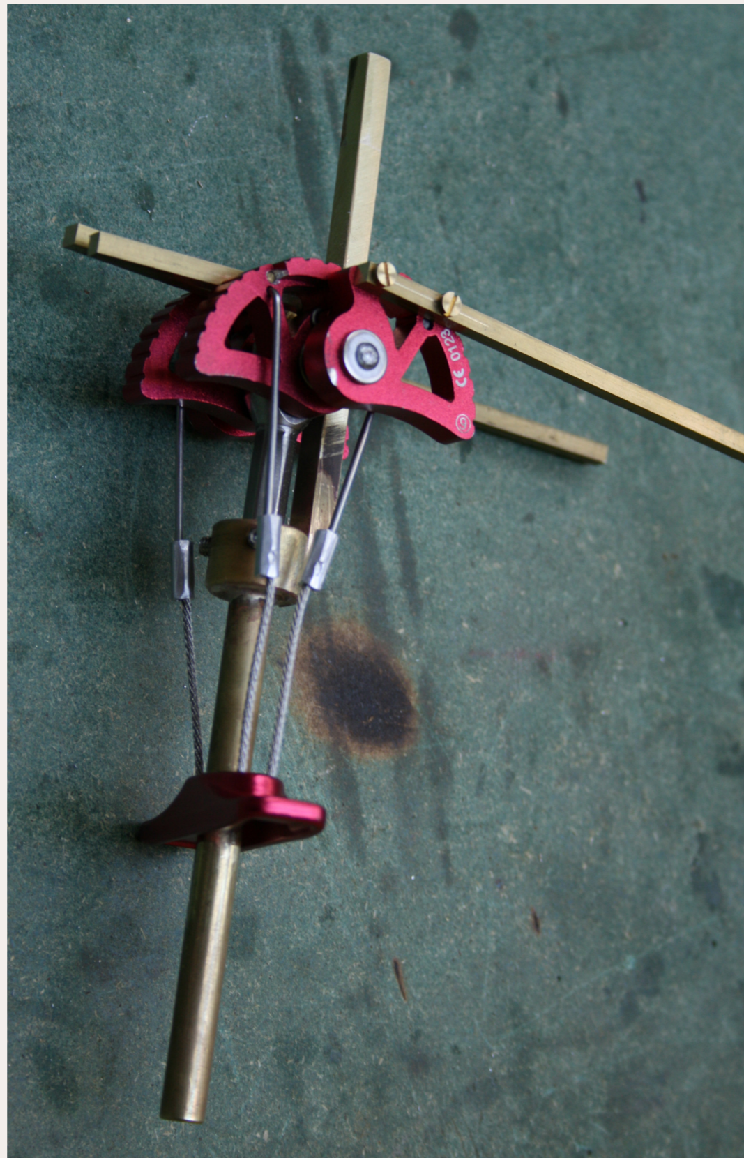
FIGURE 7.23. The new internal armature system used to position the head
