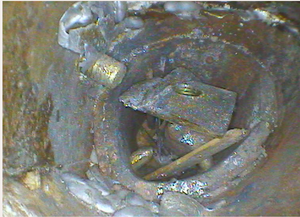
FIGURE 7.12. Endoscopic examination of the join of the modern addition to the right leg. The bronze plate, now twisted, with the hole for a thread screw is clearly visible (second phase of restoration).
