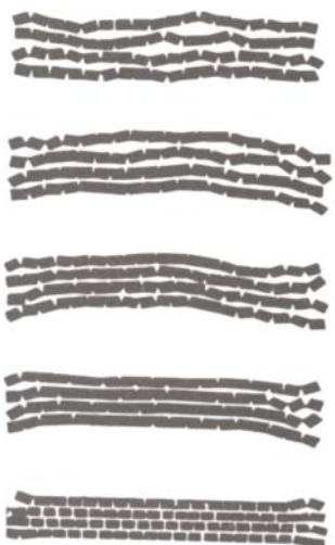
Figure 4.6. Some configurations of sheets of anhydroglucose units showing the intramolecular ordering of the polymer (Atalla 1981:172).
