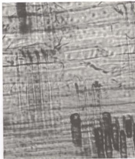
Figure 2.45 (left). Radial section of trunk wood of western red cedar, Thuja plicata Donn., showing narrow ray parenchyma cells of the wood ray and tracheids with bordered pits on the radial walls.
