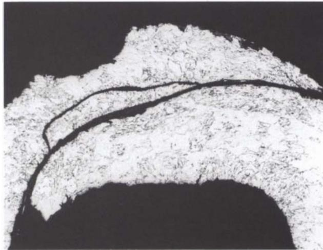
FIGURE 9. *Possible hammer scale (see arrow) lodged in crack between layers of bead from Feature 94A. Magnification  $43\times$ . Hydrogen peroxide-ammonium hydroxide etch.*
