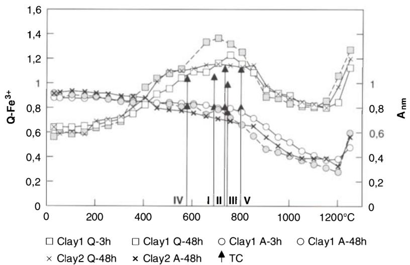
FIGURE 8. Dependence of the Mössbauer spectra measured at room temperature of Batán Grande clay 16-1 on the temperature of firing in air for 48 hours.
