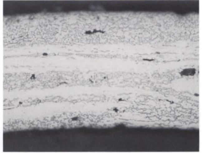
FIGURE 24. *Small fragment of a gold-platinum sintered penannular nose ring from Colombia. Etched in aqua regia. The mounted fragment measures 1.5 × 0.26 × 0.7 mm. Magnification 790×. In the collections of the Museo del Oro, Bogotá, Museum No. 4729.*
