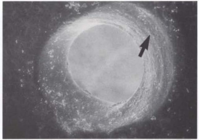
FIGURE 8. Scanning photomicrograph of the side wall, showing shallow, concentric grooves (see arrow). Magnification 59 $\times$ .
