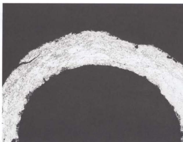
FIGURE 13. *Close-up of bead microstructure from Feature 60 showing distinct layers demarcated by thin pressure weld lines and grain elongation in different directions. Magnification 88 $\times$ . Hydrogen peroxide-ammonium hydroxide etch.*
