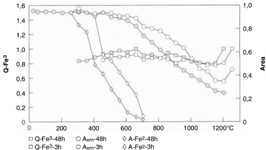
FIGURE 13. Dependence of the Mössbauer spectra of Batán Grande clay measured at room temperature on the firing temperature in air for 48 hours, following a preceding reduction at 800 °C.
