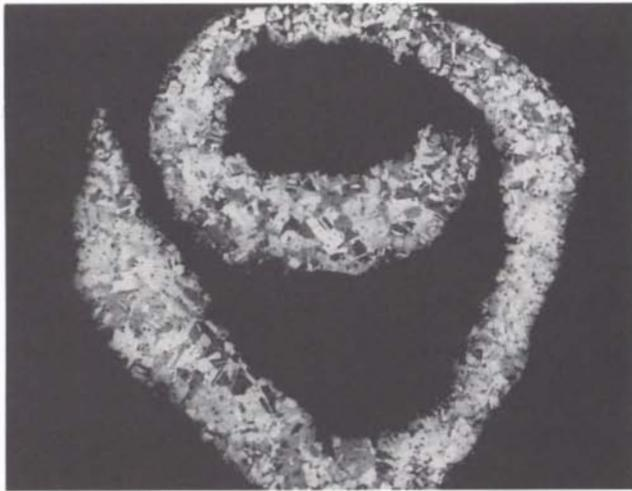
FIGURE 23. *Cross-sectional view of an end of a spiral from the Adams site. Magnification 12 $\times$ . Potassium dichromate etch.*
