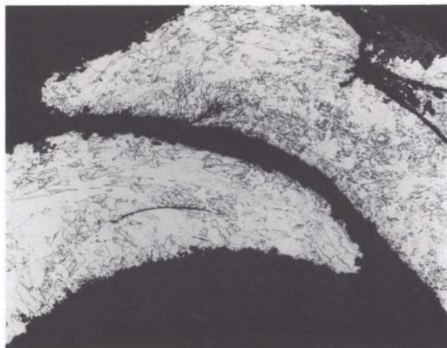
FIGURE 8. *Overlapping ends of bead from Feature 107 dating to  $670 \pm 95$  B.C.E. showing a flap of metal folded onto interior surface of bead. Magnification  $17\times$ . Hydrogen peroxide-ammonium hydroxide etch.*
