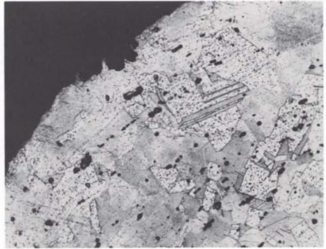
FIGURE 24. *Numerous cuprous oxides in the relatively pure copper from the Dwyer site. Magnification 72 $\times$ . Potassium dichromate etch.*
