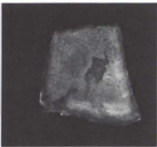
FIGURE 5. Piece of hammered silver/copper alloy sheet used in fabrication process (N<sup>o</sup> 87, WII). Lower and right edges show marks of a cutting tool. Length 1.35 cm, weight 0.41 g.
