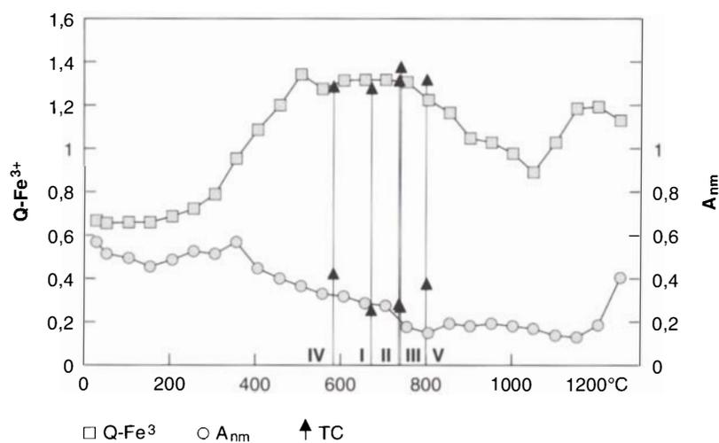
FIGURE 10. Dependence of the Mössbauer spectra measured at 4.2 K of Batán Grande clay 16-1 on the temperature of firing in air for 48 hours.
