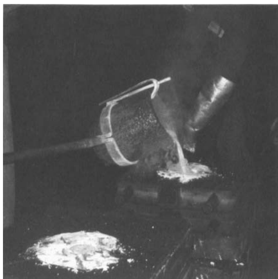
FIG. 6 Molten bronze being poured into investment mold rammed in sand.
