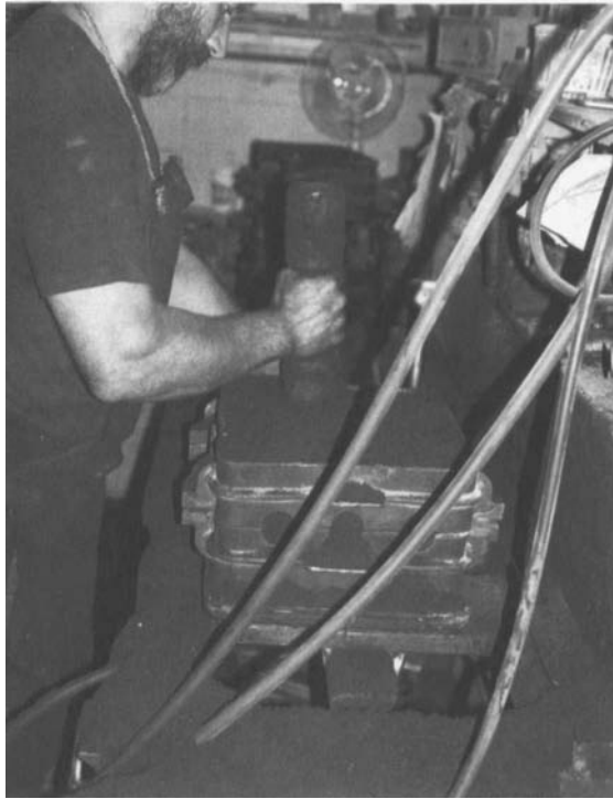
FIG. 5 Moist sand being compressed into container supporting mold.
