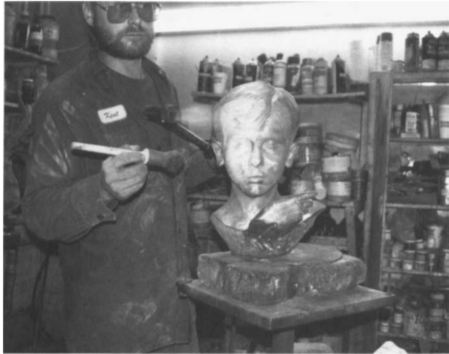
FIG. 9 Brush and blowtorch being used to achieve chemically induced patination.
