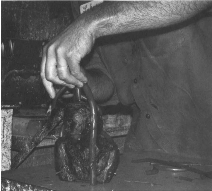
FIG. 3 Gates and vents being applied to the wax mold.
