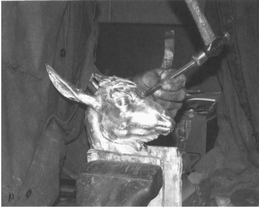
FIG. 8 Chasing tools being used to carve and texture the surface of the cast.
