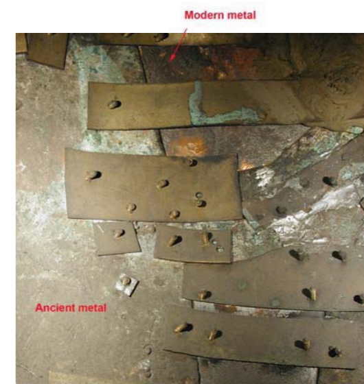
FIGURE 9.11. Interior photograph of torso taken with a hand-held digital camera showing the difference between the ancient metal and the restoration metal
