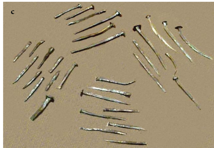
FIGURES 6.16a–c. The Minerva's internal wood support (and Carradori's iron armatures for the head and right arm) and main stucco integration (a–b); thirty-two of the forty-four fixing nails extracted during the dismantling of the sculpture (c)
