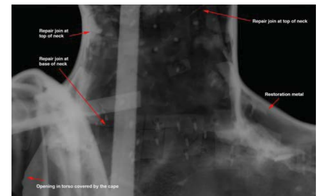
FIGURE 9.15. Radiograph of back of the neck showing the trimmed break line at the base of the neck with the straps bridging this break. There is another repaired break line at the top of the neck. The red arrow in the lower left-hand corner indicates the straight cast edge of the torso opening on the back.
