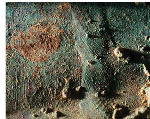
FIGURE 6.23. Protruberances marking junction of wax sheets
