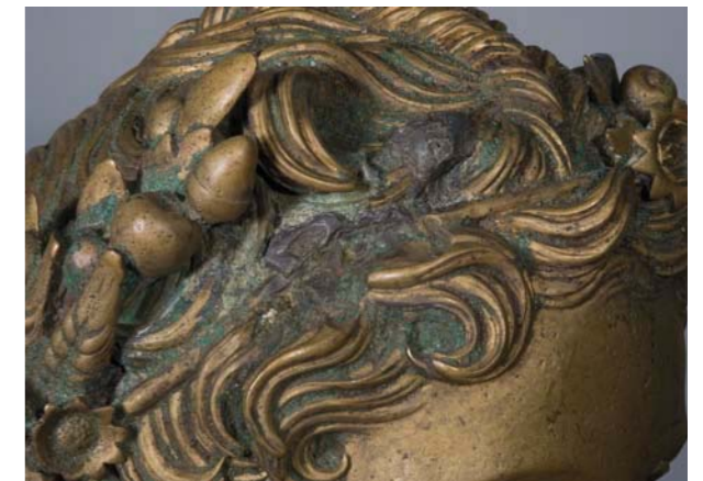
FIGURE 8.21. The Xanten Boy: green corrosion layer in the hollows of the locks of hair
