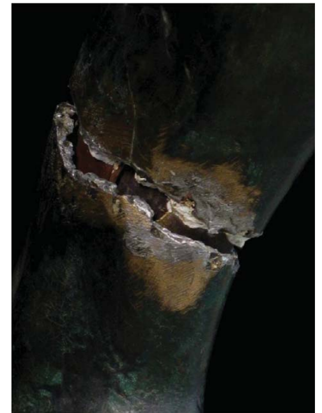
FIGURE 4.19. Apollo: detail of right ankle fracture, showing golden yellow color of exposed metal
