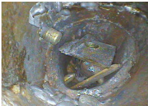
FIGURE 7.12. Endoscopic examination of the joint of the modern addition to the right leg. The bronze plate, now twisted, with the hole for a thread screw is clearly visible (second phase of restoration).
